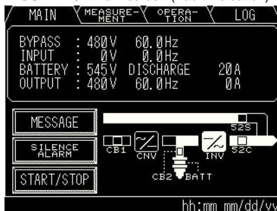
FIGURE 2.8 Main screen (Fault indication)
